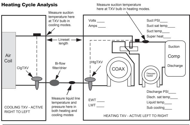
Heat of Extraction/Rejection = GPM x 500 (485 for water/antifreeze) x  $\Delta$ T Note: DO NOT hook up pressure gauges unless there appears to be a performance problem.
